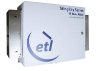
The StingRay RF over Fibre Outdoor unit (ODU) is a robust weatherproof (IP65 rated) enclosure which has been designed to be wall or post mounted close to the antenna. It can accommodate up to 10 Transmit or Receive 200 series StingRay Fibre modules.
