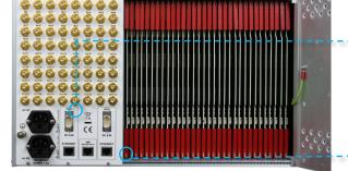
Remote control & monitoring via RJ45 Ethernet port with SNMP & web browser interface
